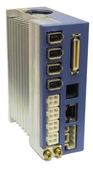
The motionCODEC<sup>™</sup> MC4 integrated drive packs 4-axis motion control and drive electronics into a trend-setting small footprint form factor measuring just 4.5" x 1.6 x 3.25". The compact size provides system designers greater flexibility in drive location within OEM equipment, minimizing cabling and EMC issues.
